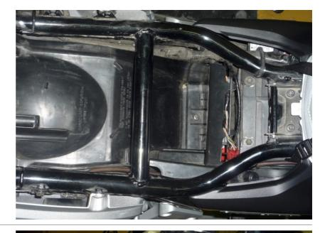
Remove the left and right frame cover below the seat.
