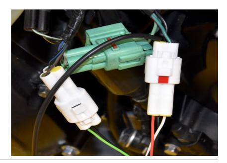
Connect the GPAT G2 Red wire to the Blue wire of the brake light switch 2-pole connector.
