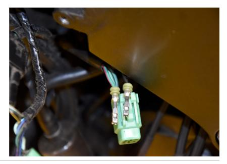
Insert the two female terminals to the smaller 3-pole plug adapter.
